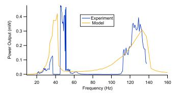
**Figure 9.** A comparison of the power output of the experiment and the predicted output of the model in response to 5.5 W of rms input power.
