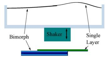
**Figure 1.** Cartoon of beam setup mimicking the experimental device. The fixed ends are approximately 20 cm apart and the overlap is approximately 10 mm. The lower detail is a zoomed in view of the joint and is not to scale with the rest of the image.
