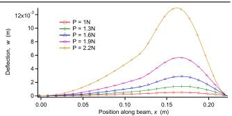
**Figure 4.** Evolution of buckled equilibrium position with axial loads between 1 and 2.2 N. Note that the right-hand side of the beam, which consists of the single-layer portion, exhibits much larger deviations from the centerline than the bimorph section. In this paper, the curve at P = 1.3 N will be used for analysis.
