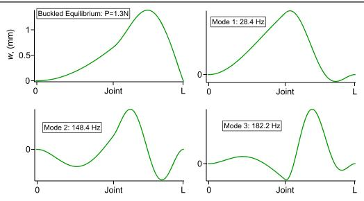
**Figure 6.** Buckled equilibrium state in terms of transverse displacement and the first three normal modes with their associated frequencies about the buckled equilibrium with axial load of 1.3 N. The horizontal axis represents the distance along the beam from 0 to *L*, while the vertical axis portrays the transverse deflection, actual for the buckled equilibrium mode and normalized for the linear modes.
