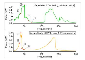
**Figure 7.** A comparison of the power output of the experiment and the predicted output of the model. Points marked as (a) through (h) will be used to compare dynamic behavior of the experimental system and the model, as shown in figure 8.
