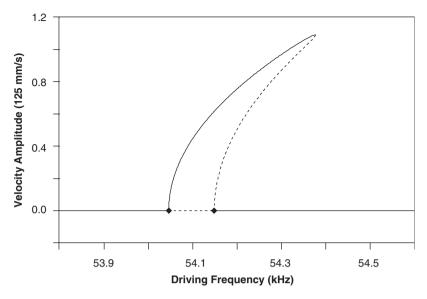
Fig. 29. Numerical frequency response curves for  $V_A = 7.6$  V. Note the hardening behavior exhibited in the system's frequency response.
