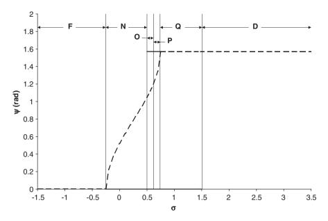
Fig. 10. Representative frequency response plot showing phase angle versus frequency detuning for Region Va ( $\gamma_3 = -0.005$ ,  $\lambda_3 = -0.010$ ) in Fig. 2.
