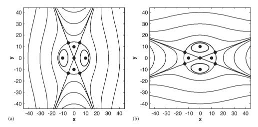
Fig. 15. Representative phase planes corresponding to the frequency (detuning) boundaries (a) OP and (b) ST where the saddle connection global bifurcations occur.
