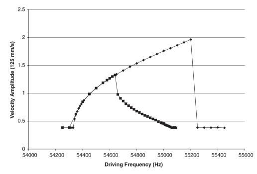
Fig. 34. Experimental frequency response curves for  $V_A = 16.6$  V. Diamonds correspond to the up sweep data points and squares to the down sweep data points. Note the mixed nonlinear behavior exhibited in the system's frequency response.
