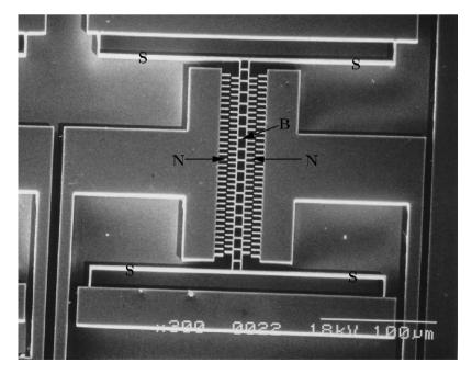
Fig. 1. A representative parametrically excited MEM oscillator. The oscillator's backbone is labeled B, S designates the mechanical beam springs, and N designates the non-interdigitated comb drives, which are used to provide the parametric excitation.
