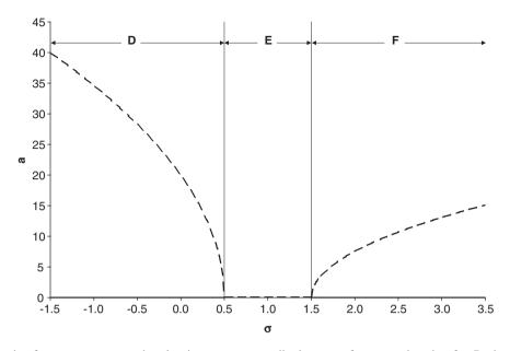
Fig. 4. Representative frequency response plot showing response amplitude versus frequency detuning for Region IIa ( $\gamma_3 = 0.005$ ,  $\lambda_3 = 0.010$ ) in Fig. 2. Note the response's mixed nonlinear characteristics.
