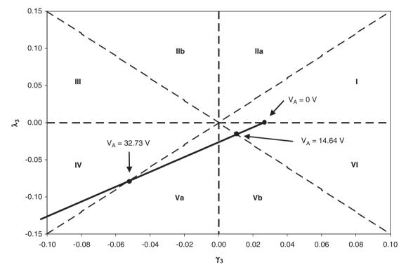
Fig. 28. Sample nonlinear parameter space showing how the system nonlinearity transitions between response regimes under a varying AC voltage amplitude for the device presented in Table 2.
