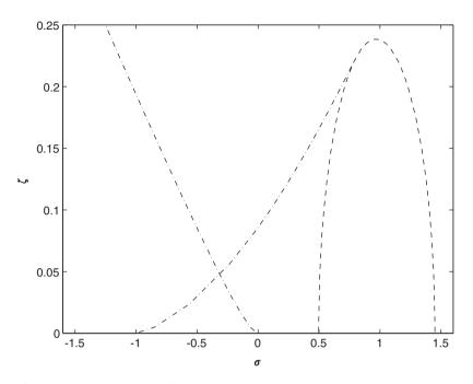
Fig. 23. Bifurcation sets for the parameters corresponding to Region IV. The no-motion state is unstable inside the dashed curve, while the dot-dashed lines show bifurcation sets for the saddle-node bifurcations of the symmetric periodic orbits.
