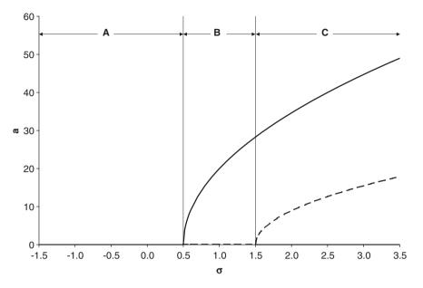
Fig. 3. Representative frequency response plot showing response amplitude versus frequency detuning for Region I ( $\gamma_3 = 0.005$ ,  $\lambda_3 = 0.005$ ) in Fig. 2. Note the response's hardening nonlinear characteristics. Also note that here, as well as in Figs. 4–14, solid lines indicate stable response branches and dashed lines unstable response branches.
