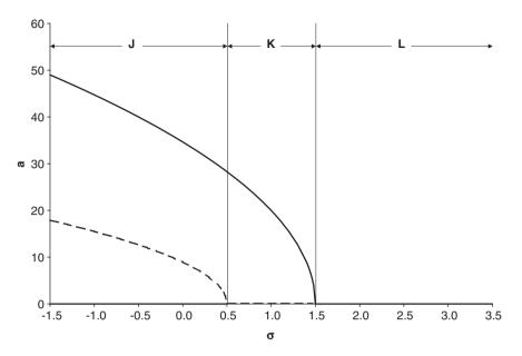
Fig. 6. Representative frequency response plot showing response amplitude versus frequency detuning for Region III ( $\gamma_3 = -0.005$ ,  $\lambda_3 = 0.005$ ) in Fig. 2. Note the response's softening nonlinear characteristics.
