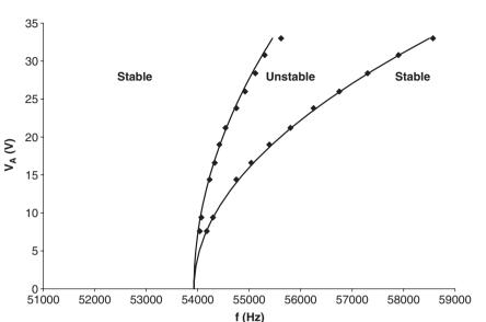
Fig. 27. Linear stability chart in the AC excitation voltage amplitude  $(V_A)$  versus excitation frequency (f) parameter space for an undamped MEM oscillator with system parameters as specified in Table 2. Experimentally derived instability points are also shown. Note that in each case the noted stability corresponds to the trivial solution.
