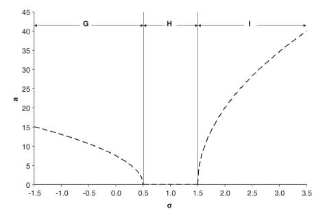
Fig. 5. Representative frequency response plot showing response amplitude versus frequency detuning for Region IIb ( $\gamma_3 = -0.005$ ,  $\lambda_3 = 0.010$ ) in Fig. 2. Note the response's mixed nonlinear characteristics.
