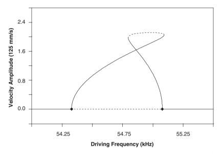
Fig. 30. Numerical frequency response curves for  $V_A = 16.6$  V. Note the mixed nonlinear behavior exhibited in the system's frequency response.
