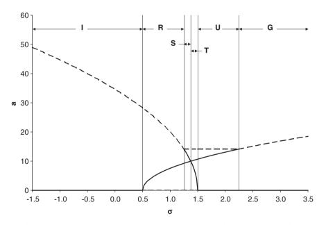
Fig. 11. Representative frequency response plot showing response amplitude versus frequency detuning for Region Vb ( $\gamma_3 = 0.005$ ,  $\lambda_3 = -0.010$ ) in Fig. 2. Note the response's mixed nonlinear characteristics.
