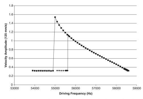
Fig. 35. Experimental frequency response curves for  $V_A = 33.0$  V. Diamonds correspond to the up sweep data points and squares to the down sweep data points. Note the softening behavior exhibited in the system's frequency response.
