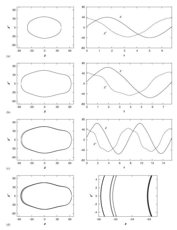
Fig. 22. Stable solutions for parameters as in Fig. 21 and with forcing  $\sim \cos \Omega \tau$ : (a) symmetric periodic orbit for  $\sigma = -1.5$ ; (b) asymmetric periodic orbit for  $\sigma = -3.85$ ; (c) period doubled orbit for  $\sigma = -3.895$ ; (d) chaotic solution for  $\sigma = -3.90235$ , with right panel zoomed in. The timeseries in (a), (b), and (c) show one period.
