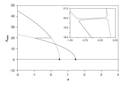
Fig. 20. Bifurcation diagram showing the maximum value of the displacement ( $z_{max}$ ) for  $\zeta = 0.001$  and other parameters as described in the text. In this and other bifurcation diagrams, diamonds, squares, and triangles indicate crossing the boundary of an Arnold tongue, period-doubling, and symmetry-breaking pitchfork bifurcations, respectively. Furthermore, solid and dashed lines represent stable and unstable solutions, respectively.
