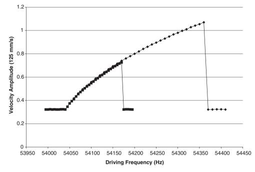
Fig. 33. Experimental frequency response curves for  $V_A = 7.6$  V. Diamonds correspond to the up sweep data points and squares to the down sweep data points. Note the hardening behavior exhibited in the system's frequency response.
