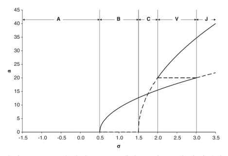
Fig. 13. Representative frequency response plot showing response amplitude versus frequency detuning for Region VI ( $\gamma_3 = 0.005$ ,  $\lambda_3 = -0.005$ ) in Fig. 2. Note the response's quasi-hardening nonlinear characteristics.
