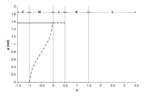
Fig. 8. Representative frequency response plot showing phase angle versus frequency detuning for Region IV ( $\gamma_3 = -0.005$ ,  $\lambda_3 = -0.005$ ) in Fig. 2.
