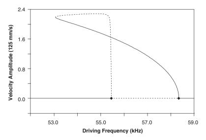
Fig. 31. Numerical frequency response curves for  $V_A = 33.0$  V. Note the softening (quasi-softening) behavior exhibited in the system's frequency response.
