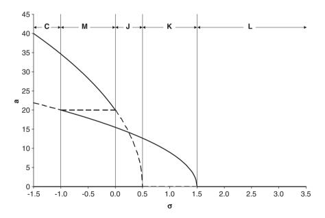
Fig. 7. Representative frequency response plot showing response amplitude versus frequency detuning for Region IV ( $\gamma_3 = -0.005$ ,  $\lambda_3 = -0.005$ ) in Fig. 2. Note the response's quasi-softening nonlinear characteristics.
