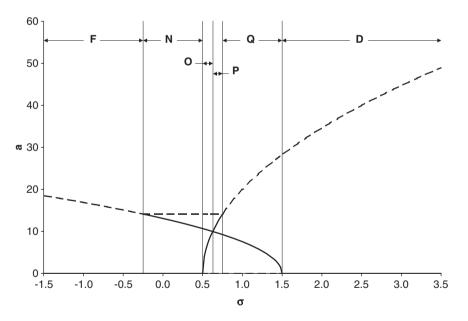
Fig. 9. Representative frequency response plot showing response amplitude versus frequency detuning for Region Va ( $\gamma_3 = -0.005$ ,  $\lambda_3 = -0.010$ ) in Fig. 2. Note the response's mixed nonlinear characteristics.
