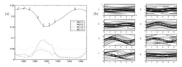
Figure 2: (a) RMS modal velocities for several wavenumbers, and (b) midplane streamwise-velocity contours for one representative cycle from the direct numerical simulations.
