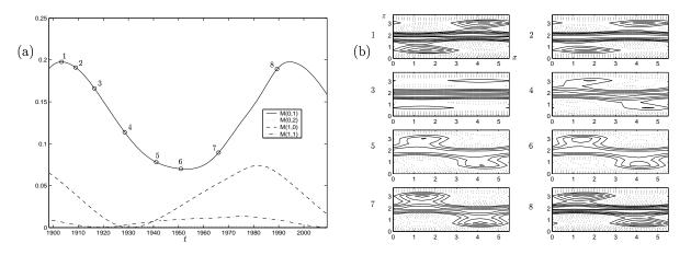
Figure 3: (a) RMS modal velocities for several wavenumbers, and (b) midplane streamwise-velocity contours for one period for the model at Re = 400.
