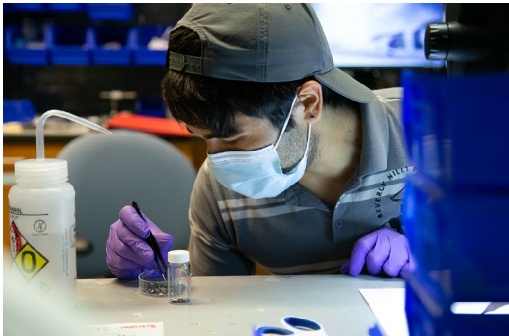
Brenden R. Ortiz, postdoctoral researcher in Stephen Wilson's materials lab at UCSB, separates newly grown crystals, the result of placing the mixed elements in a steel capsule, heating them to one thousand degrees Celsius, then slowly cooling them to five hundred degrees over a two-week period. Here, he begins the laborious task of using tweezers and solvent to separate the crystals from unwanted residue.
