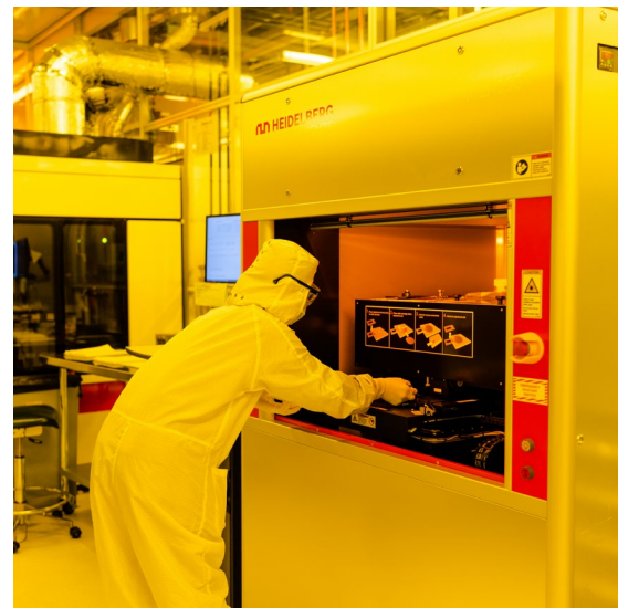
Engineering the small (from top): a transmitter photonic circuit made by the Bowers group in the Nanofab; a technician works at a station in the amber-lit lithography bay, where light-sensitive materials are used to transfer patterns onto wafers to guide fabrication.
