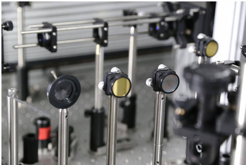
A series of lenses and optical relays direct the laser light to the sample.
