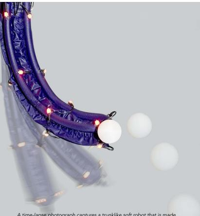
A time-lapse photograph captures a trunklike soft robot that is made of fabric, incorporates fabric "muscles," and is controlled by Koopman Operating Theory tossing a ping pong ball.
